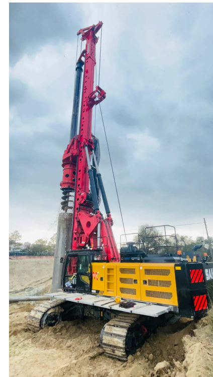
SR285MV in Turkey with short auger and long casing
