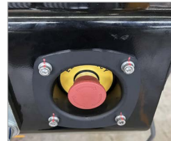
Emergency stop switch around the machine
